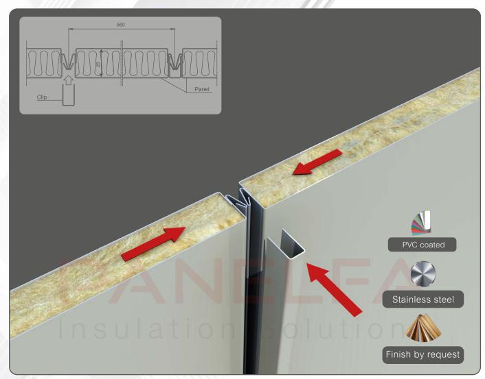
The CLIP 25 Panel has been designed to achieve the requests of the new constructions for lining application. The features of this panel allow a better adaptation to the space and a fast installation.
