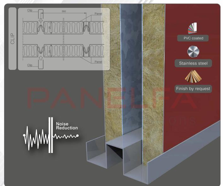
The clip double Panel 25 NR has been designed to achieve the requests of the new constructions. The features of these products offers a high noise reduction, adapting in this way to the requirements that in the field of comfort are in force in modern constructions.
